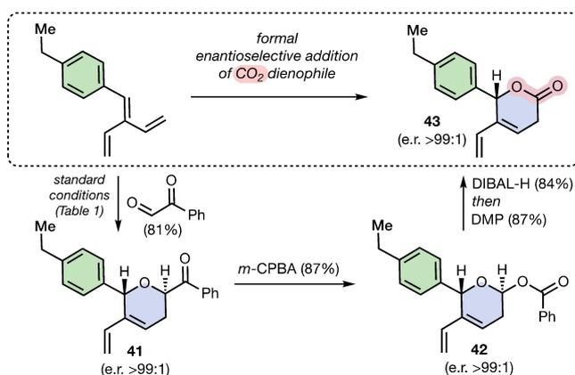
**Scheme 3.** Phenylglyoxal as a synthetic equivalent of a CO<sub>2</sub> dienophile in an enantioselective ODA reaction.
