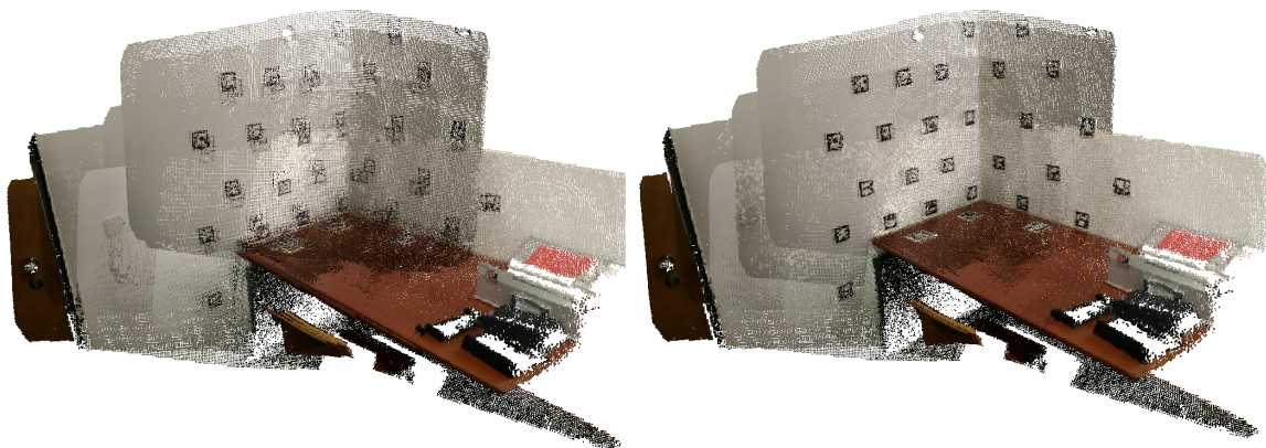
Figure 4. Merged point cloud coloured with texture obtained from images: (left) before optimization; (right) after optimization.
