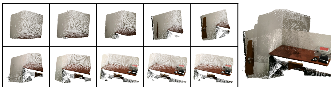
Figure 1. Example of registration of several point 3D point clouds to create a complete 3D model.
