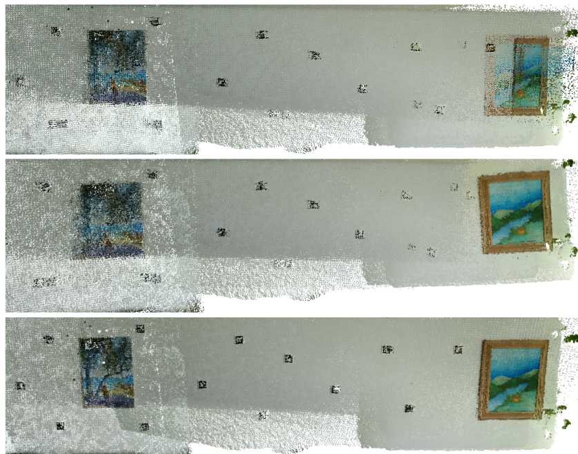
Figure 20. MeetingRoom dataset coloured with texture obtained from original images (detail 1): (top) Google Tango; (middle) ICP; (bottom) Our approach.
