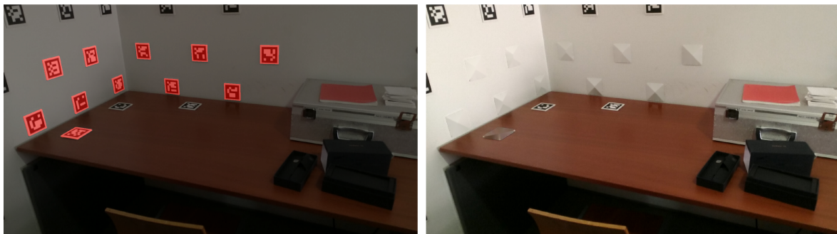
Figure 8. Example dataset image inpainting: (left) mask used for marker removal; (right) results of Navier-Stokes-based inpainting from OpenCV.
