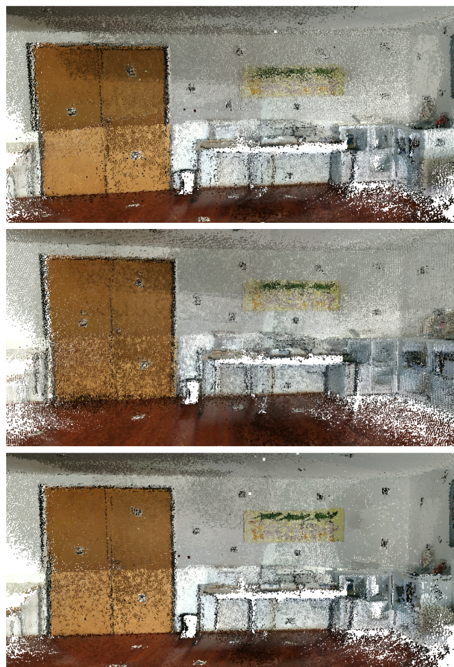
Figure 21. MeetingRoom dataset coloured with texture obtained from original images (detail 2): (top) Google Tango; (middle) ICP; (bottom) Our approach.
