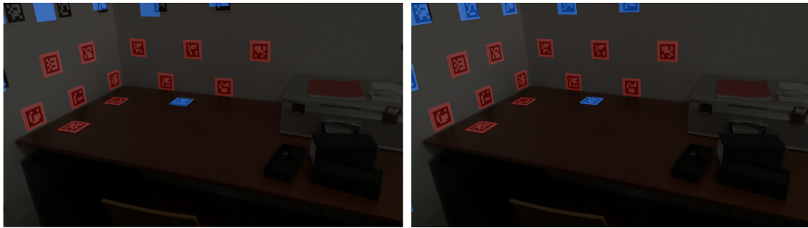
Figure 13. Masks obtained from aruco marker detection in red and masks obtained from projections from other cameras (cross-Inpainting) in blue: (left) before optimization; (right) after optimization.
