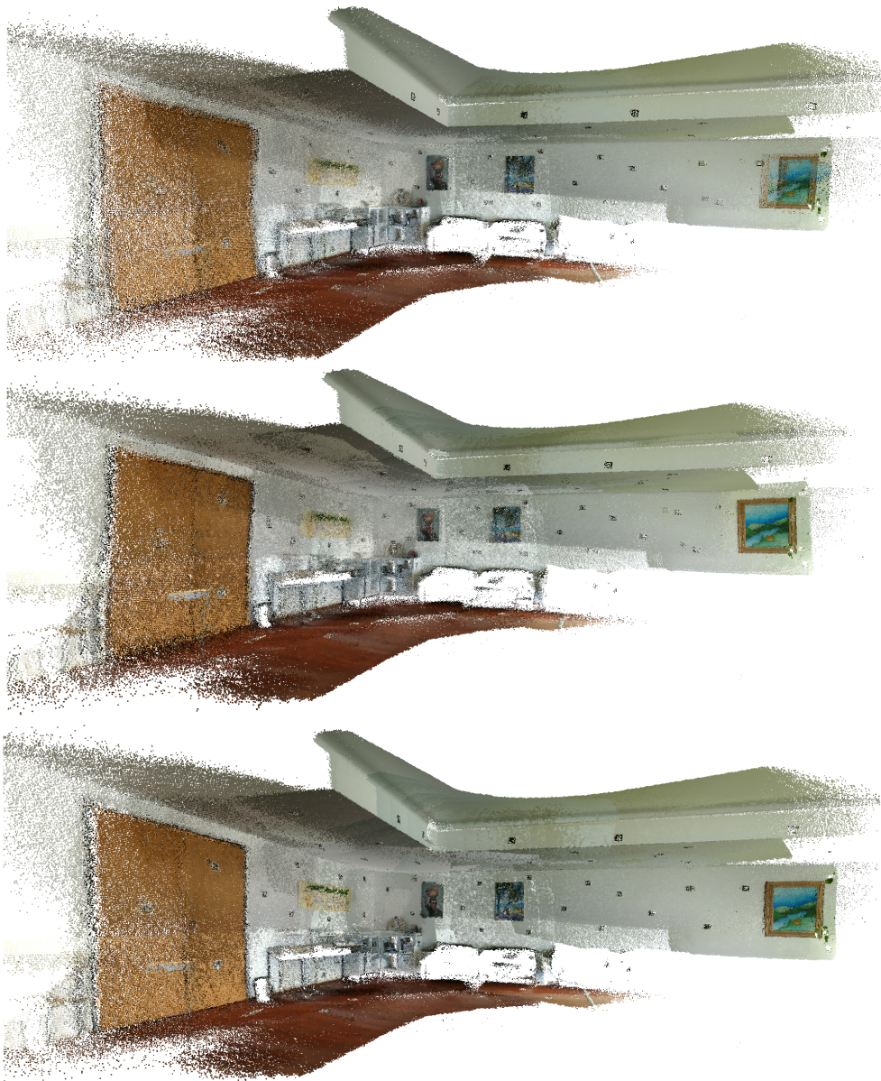
Figure 19. MeetingRoom dataset coloured with texture obtained from original images: (top) Google Tango; (middle) Iterative Closest Point (ICP); (bottom) Our approach.
