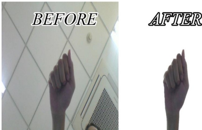
Fig. 4. Original image and its segmentation with removed background by Otsu's method and enhanced by technical expert.
