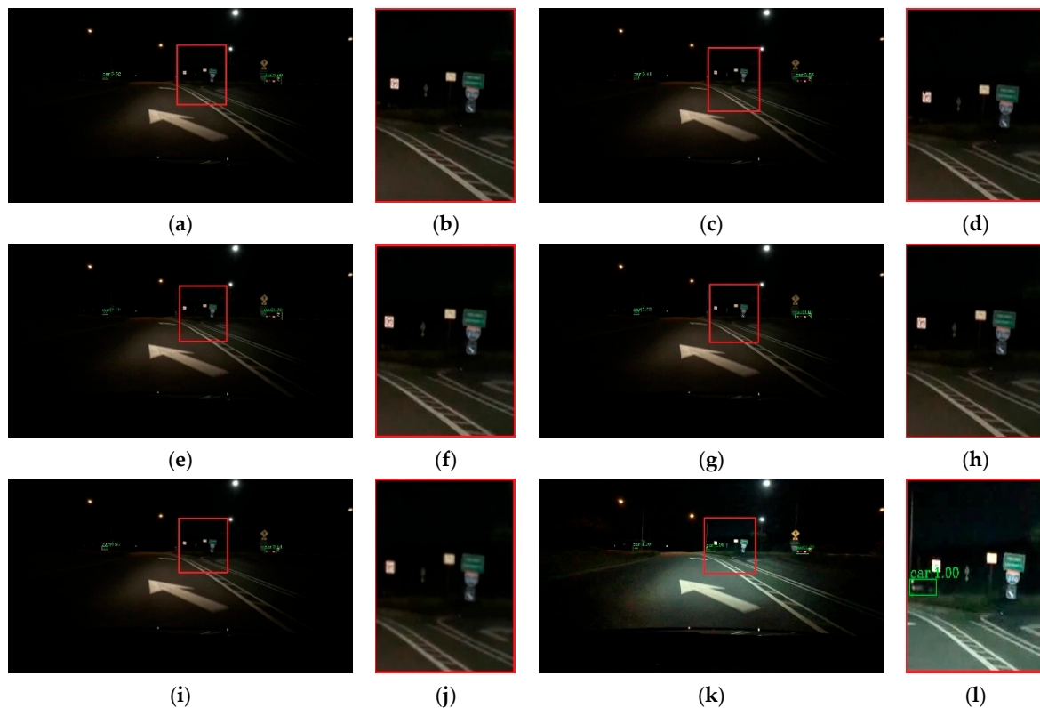
Figure 7. Detection results of dark scene. (a) faster R-CNN, (c) Cascade R-CNN, (e) Mask R-CNN, (g) RetinaNet, (i) SSD, (k) ours. (b,d,f,h,j,l) represent the red area of (a,c,e,g,i,k) respectively.
