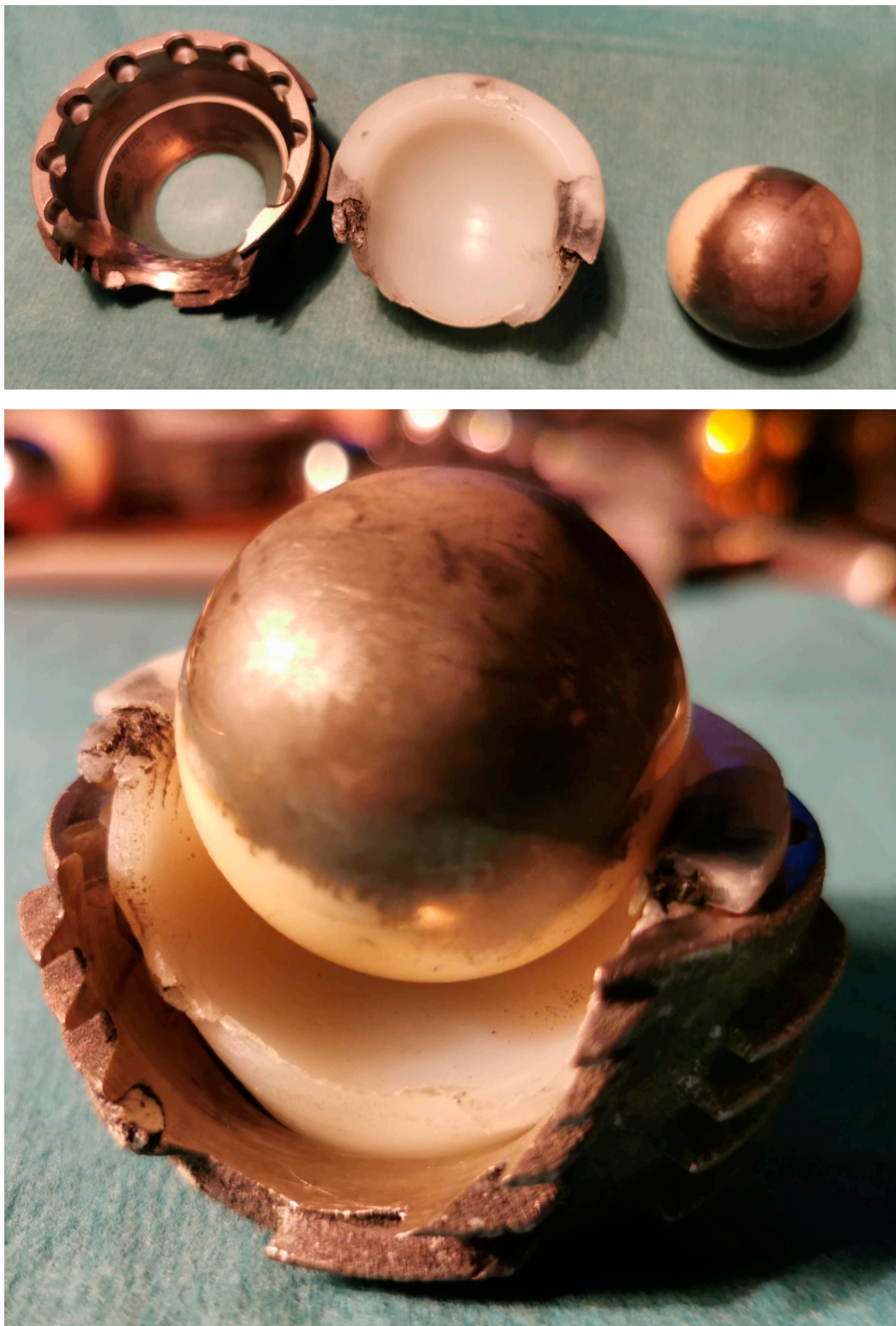
Figure 5. An example of the acetabular cup grinding and its UHMWPE insert by \text{Al}_2\text{O}_3 ceramic head during decades-long weight bearing.
