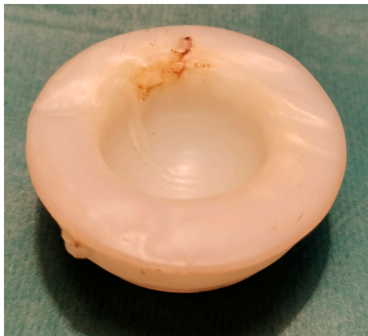
Figure 3. Creep and wear leading to deformation of the acetabular UHMWPE insert.
