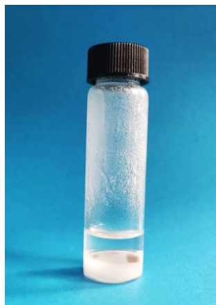
Figure S5. Limited dissolution of LiFSI in \text{PhCF}_3 .
