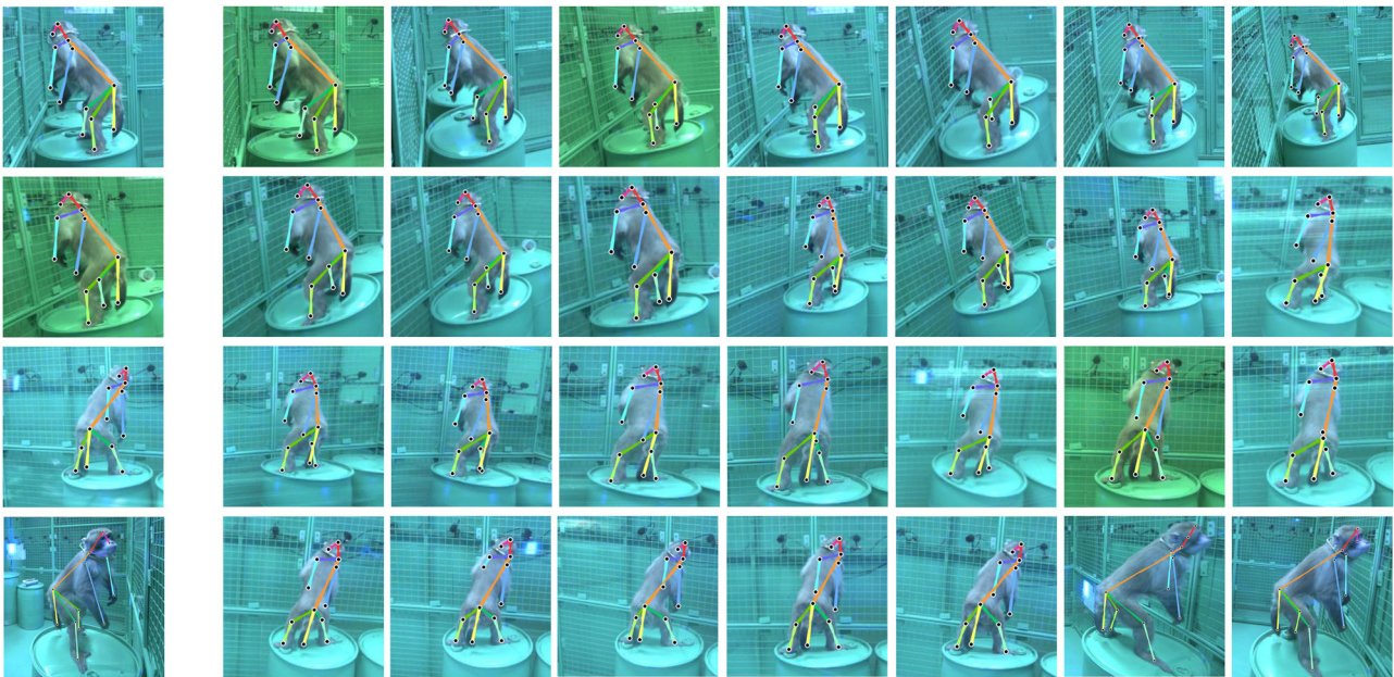
Fig. 9 Multiview augmentation. OpenMonkeyStudio leverages multiview geometry to augment the annotated data across views. The three images in the left most column are manually annotated and the 2D pose of the rest images are automatically augmented by 3D reconstruction and its projection.
