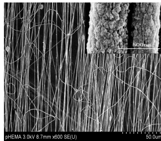
Aligned nanofibers by MPEM (1.0 wt %)
