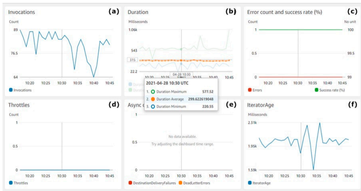
Figure 9. AWS Lambda performance metrics. (a) Invocations, (b) duration, (c) error count and success rate (%), (d) throttles, (e) async delivery errors, (f) iterator age.
