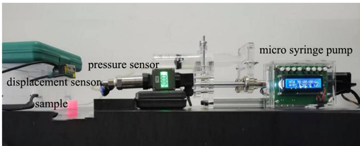
Figure 6. Physical diagram of diaphragm flip quasi-static test rig.
