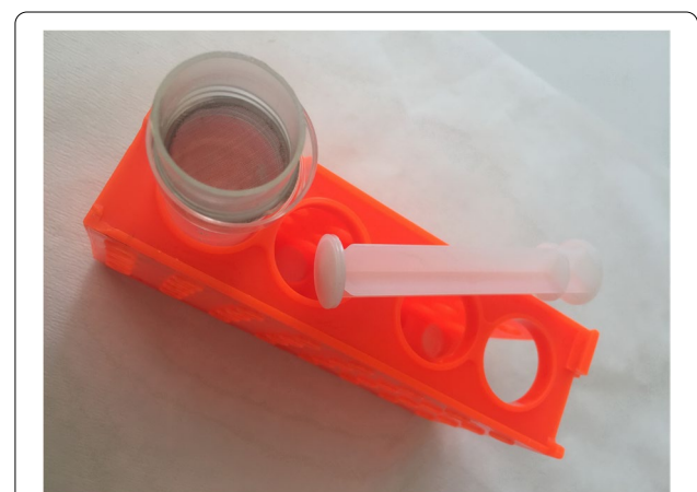
Fig. 6 Image of the sieving device ( 100\ \mu\text{m} cell strainer) for pulverization and filtration of ALN tissue to obtain cell suspension free from fat and connective tissue (for details see Methods)
