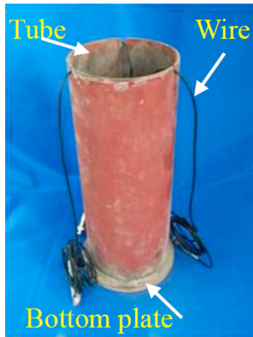
Figure 11. The steel tube.
