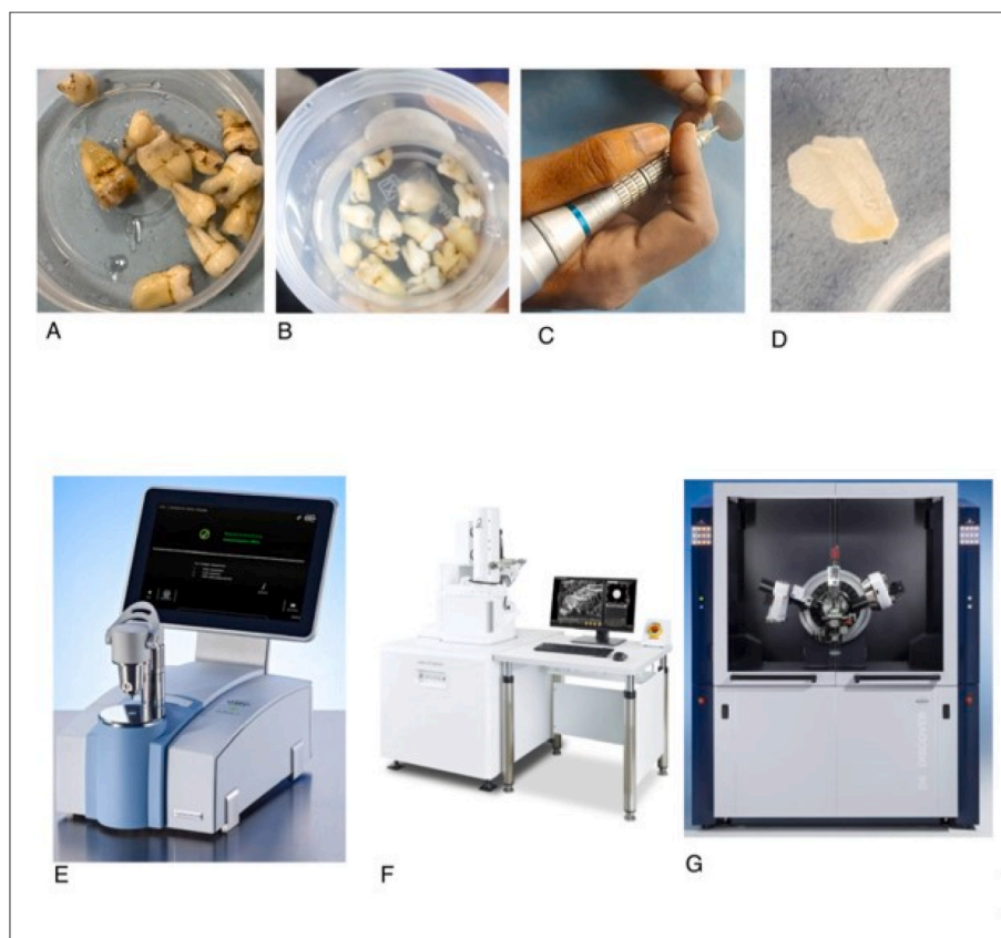
Fig. 1. Methodology A) Selection of teeth; B) Immersion in 10 % HCl; C) Sectioning of test teeth; D) Sectioned tooth; E) FTIR machine; F) SEM machine; G) XRD machine.
