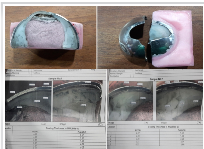
Figure 4: Spectro-analysis showing the wear of polyethylene and thickness of outer metallic dome.
