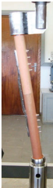
FIGURE 3: Apparatus for applying concomitantly compression and flexion to the specimens. Angle between the load application line and the specimen centerline: 9^\circ .
