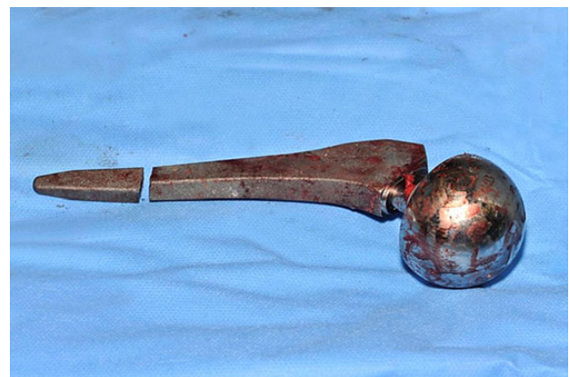
Figure 4: Broken stem in Case 1.
