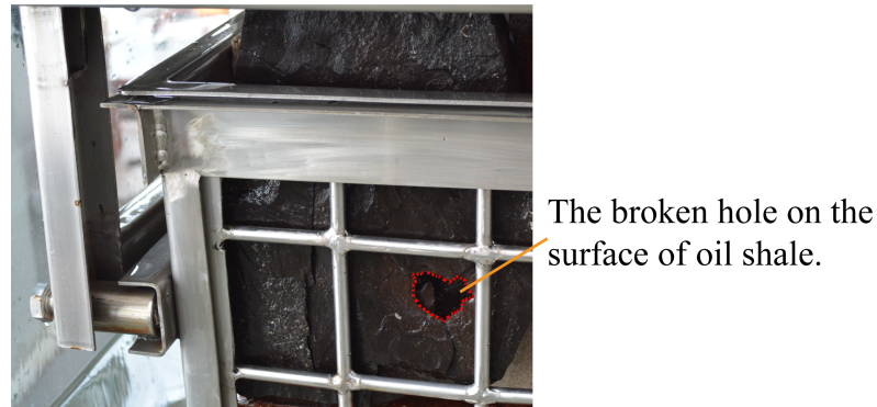
Fig 15. Broken oil shale sample by the direct water jet which is perpendicular to the bedding of oil shale.
