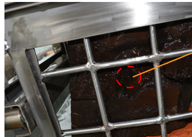
Fig 20. Broken oil shale sample by the pulsed water jet which is perpendicular to the bedding of oil shale.
