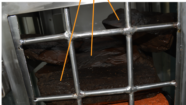
Fig 19. Broken oil shale sample by the pulsed water jet which is parallel to the bedding of oil shale. (A) The pulsed water jet is produced by the self-excited oscillation pulsed jet nozzle. (B) The broken oil shale sample by the pulsed water jet.
