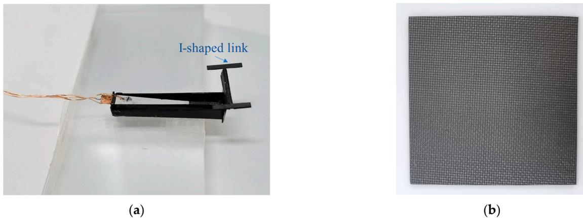
Figure 7. (a) Experimental product of miniature piezoelectric drive squama deformation mechanics; (b) squama.
