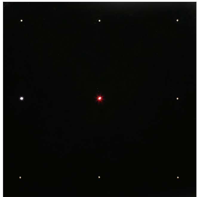
Figure 2: Photograph of orthoptek instrument. It has three rows of LEDs of each each and central one is red
