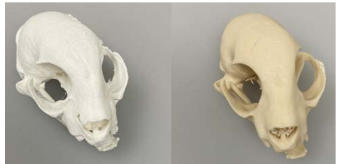
Figure 1. FDM prints of a deformed domestic cat skull using PLA- (left) and PHBHHx- (right) based filaments.
