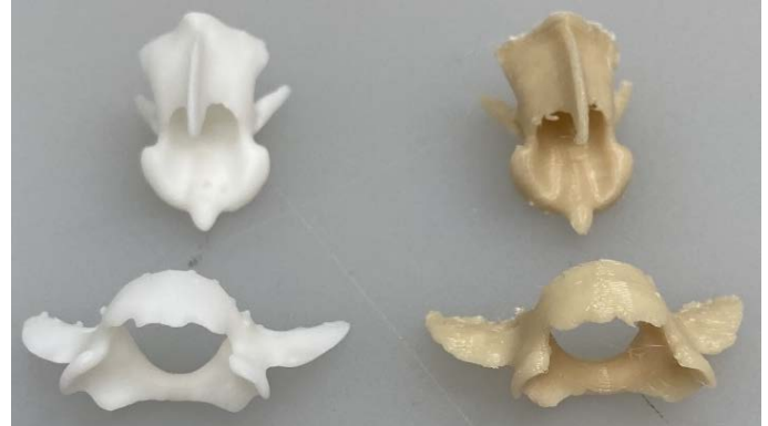
Figure 4. Improved PHBHHx- (right) based filament print quality of vertebrae samples, compared to standard SLA prints (left).
