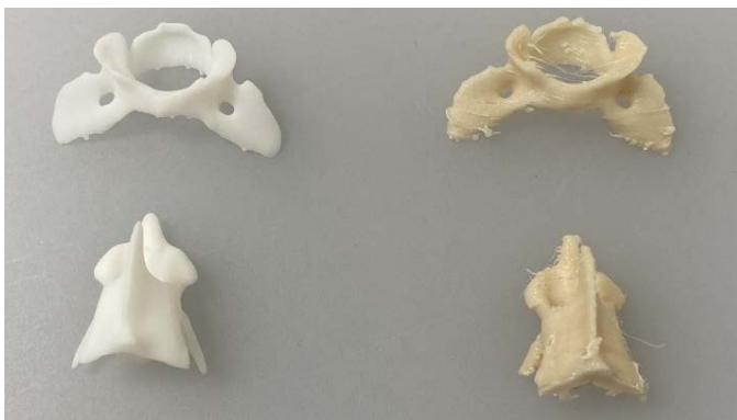
Figure 3. Imperfect print quality in PHBHHx- (right) based filament printing of small parts due to improper print parameter optimization, in comparison to standard SLA prints (left).
