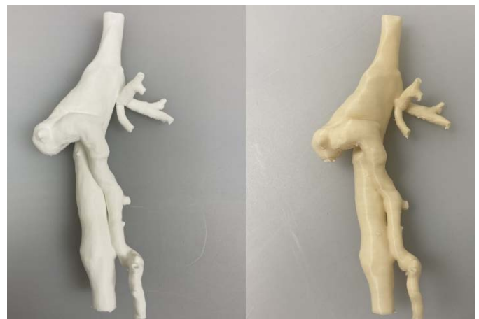
Figure 2. FDM prints of an aorta assembly using PLA- (left) and PHBHHx- (right) based filaments.
