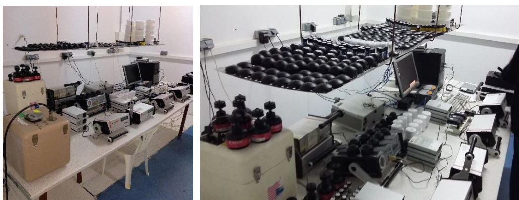
Figure 2. Radon devices inside Room1 (LNR: Laboratory of Natural Radiation).
