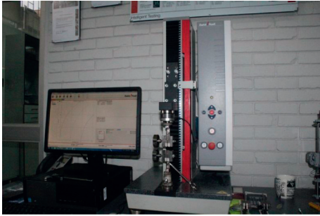
FIGURE 1: Material testing machine BT1-FR0.5TS.D14 (Zwick GmbH & Co.KG), with which the tensile measurements of all suture materials evaluated were performed.
