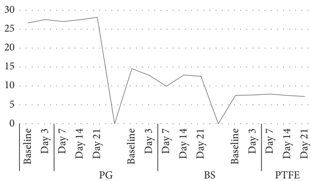
FIGURE 2: Tensile strength of various absorbable and nonabsorbable sutures according to immersion time in synthetic saliva. The tensile strength values are means expressed in Newtons. PG: polyglactin, BS: black silk, PTFE: polytetrafluoroethylene (Teflon).
