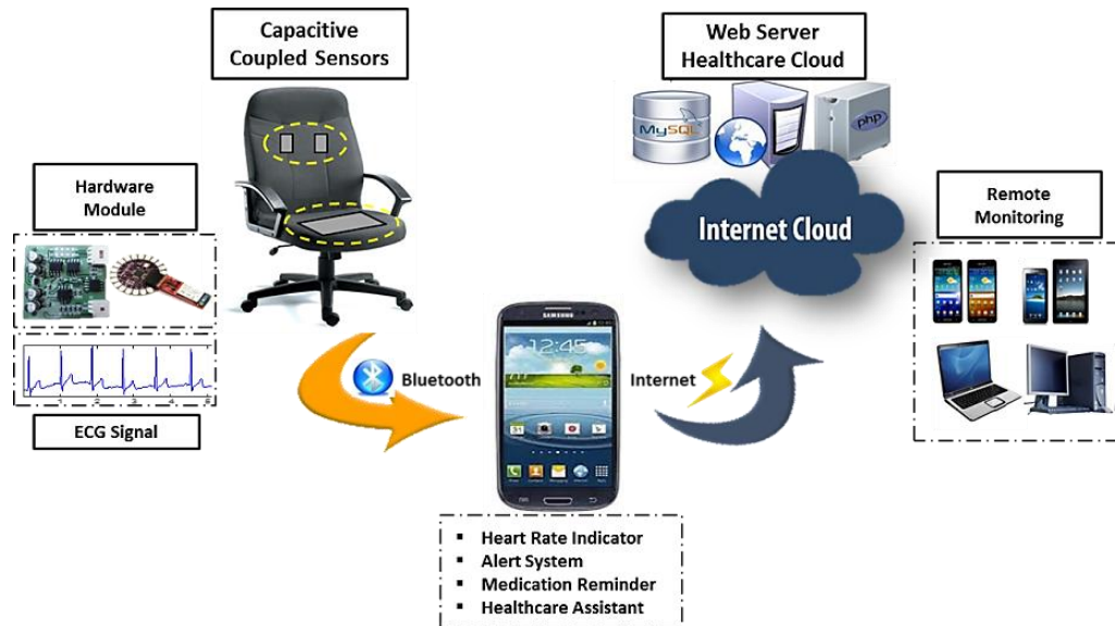
Figure 3. System design of mobile healthcare and cloud-based service for noncontact ECG monitoring system, which consists of a data acquisition module, a mobile system, and a cloud computing Web server module.
