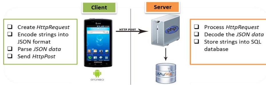
Figure 9. Client-server model. The clients request and receive service from the centralized server.
