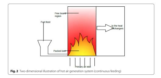
are negligible and the thermal Biot number should be less than 0.1 (Bi < 0.1) (Incroprera and Dewitt 2002). Biomass is considered as a composite of moisture, volatile, char and ash. Combustion processes can be divided into 4 sub-processes, which are consisting as follows;
