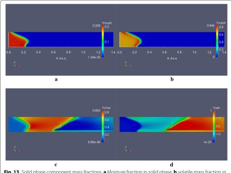
**Fig. 13** Solid phase component mass fractions. **a** Moisture fraction in solid phase, **b** volatile mass fraction in solid phase, **c** char mass fraction at solid phase, **d** ash mass fractions
