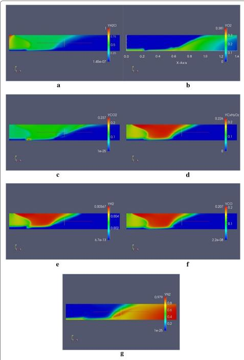
**Fig. 14** Gas component mass fractions of packed bed at steady state. **a**  $H_2O$  mass fractions, **b** oxygen  $(O_2)$  mass fractions, **c** carbondioxide  $(CO_2)$  mass fractions, **d**  $C_xH_yO_z$  mass fractions, **e** hydrogen  $(H_2)$  mass fractions, **f** carbonmonoxide (CO) mass fractions, **g** nitrogen  $(N_2)$  mass fractions
