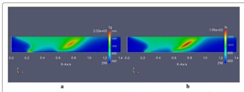
**Fig. 7** Gas phase and solid phase temperature of packed bed at steady state. **a** Temperature of gas phase (K), **b** temperature of solid phase (K)
