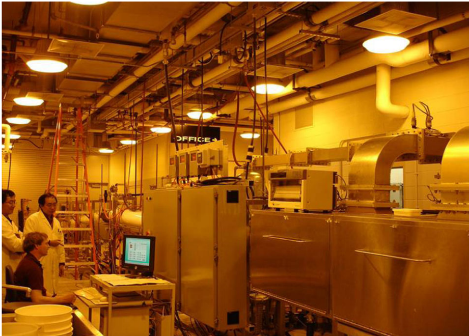
Figure 9—2nd generation pilot-scale microwave sterilization system at Washington State University.
