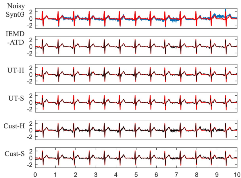
Fig 9. Waveforms of denoised ECGs for Syn03 with EMG noise at 5 dB in the 5 denoising methods.
