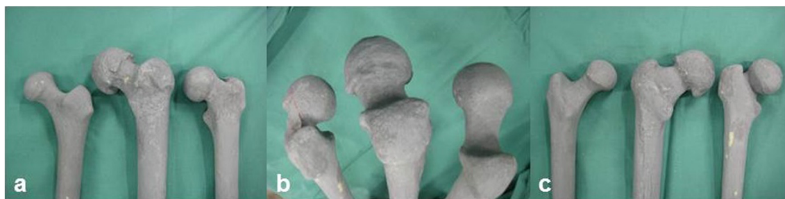
Figure 2 Head/neck morphology of the three types of synthetic femurs used in this study. Anterior (a), top (b), and posterior (c) view: normal configuration, osteophytes, slipped epiphysis (right to left).
