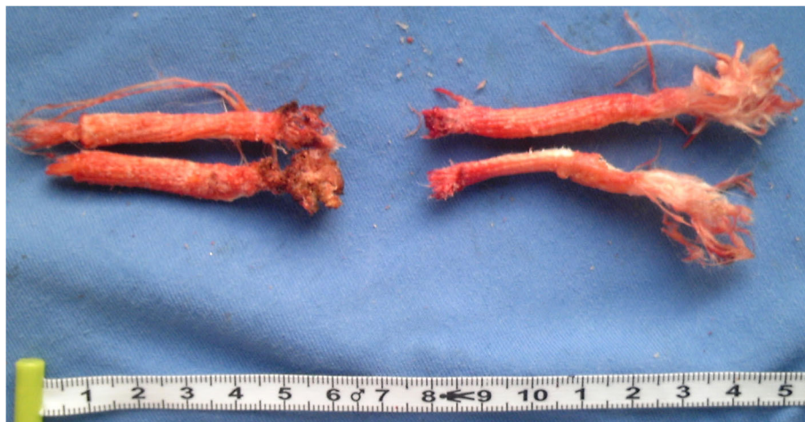
Fig. 5 The LARS device was rough and worn with visible polyethylene terephthalate debris
