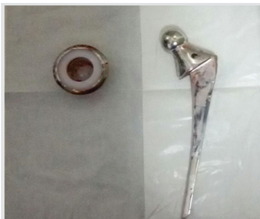
Figure 4: Intraoperative photograph of dissociated components of the prosthesis— outer head with polyethylene liner (left side) and inner headstem one piece component (right side).
