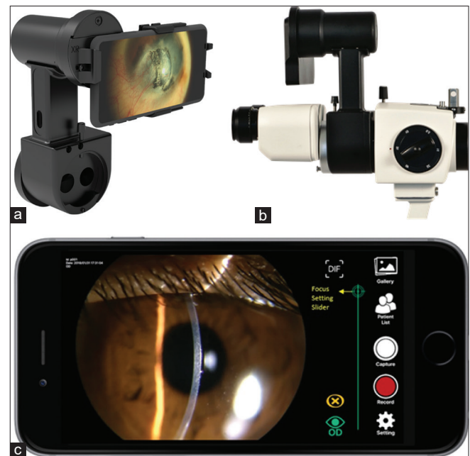
Figure 2: (a) Hardware Design of Anterior imaging Module (AIM). (b) AIM mounted on a conventional slit-lamp. (c) Anterior segment imaging on AIM
