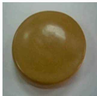
Figure 5. Color photograph of bloated iron-rich glass-ceramic sample as described in [14].
