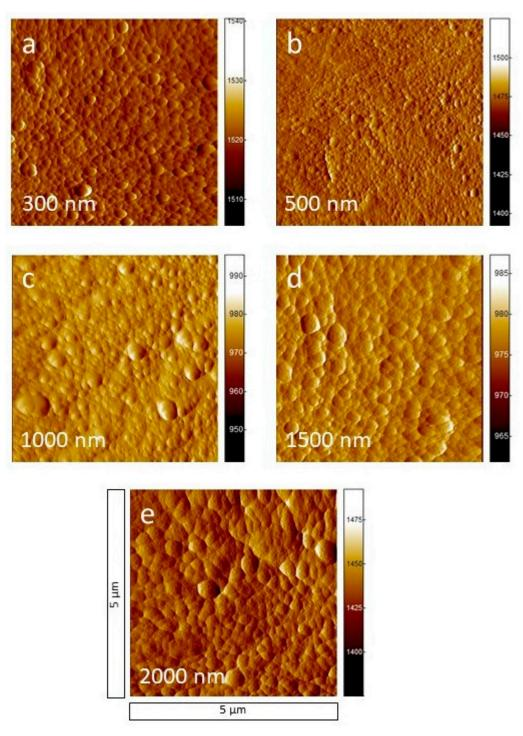
**Figure 4.** AFM measurements for PA6 samples (**a**–**e**) coated with thick a-C:H layers from (**a**) 300 up to (**e**) 2000 nm. The image size is 5  $\mu$ m × 5  $\mu$ m.
