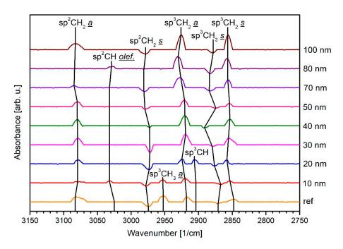
**Figure 7.** DRIFT spectra of the analyzed PA6 samples coated with thin a-C:H up to 100 nm in 10 nm steps starting from the  $O_2$  plasma-treated reference. The measurement series is applied from below to above with increasing layer thickness.
