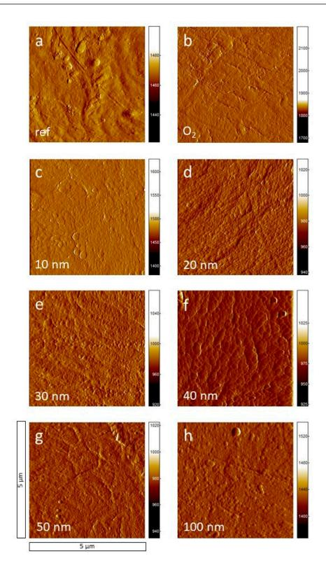
**Figure 3.** AFM images of the raw PA6 (**a**), the O<sub>2</sub> plasma-treated PA6 (**b**) samples, and PA6 samples coated with thin a-C:H layers of various thickness (10 to 100 nm, **c**–**h**). The image size is 5  $\mu$ m × 5  $\mu$ m.
