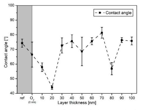
**Figure 5.** Contact angle measurements for the PA6 samples: shown are raw and O<sub>2</sub> plasma-treated PA6 as well as thin a-C:H layers up to 100 nm (the dashed line only indicates the trend).
