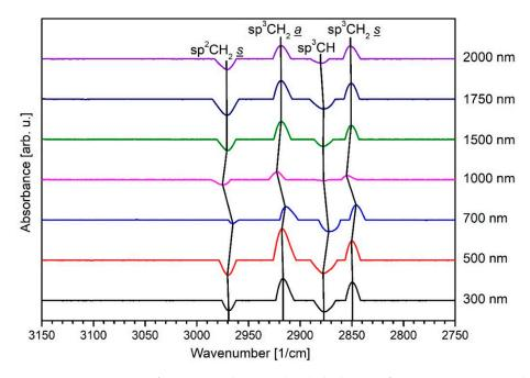
**Figure 8.** DRIFT spectra for PA6 samples coated with thick a-C:H from 300 to 2000 nm with increasing layer thickness from below.
