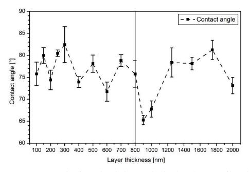
**Figure 6.** Contact angles of amorphous hydrogenated carbon (a-C:H) coatings of layer thicknesses from 100 to 2000 nm on PA6 samples (the dashed line only indicates a trend).
