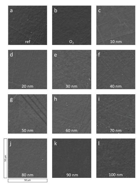
**Figure 1.** SEM surface images of PA6 samples coated with thin a-C:H layers from 10 to 100 nm in 10 nm steps (**c**–**l**). Additionally, the reference (**a**) and the O<sub>2</sub> plasma-treated PA6 sample (**b**) are added.
