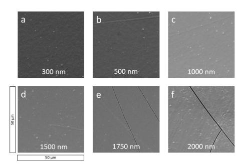
**Figure 2.** SEM analysis of thick a-C:H layers on PA6 (**a**–**f**). Thickness varies from (**a**) 300 to (**f**) 2000 nm, arranged in increasing layer thickness.
