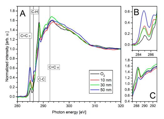
**Figure 10.** C K-edge NEXAFS measurements for PA6 coated with thin layers of a-C:H: (**A**) shows the full spectra; (**B**,**C**) present detailed photon energy intervals for carbon relevant peaks. (**B**): 283.00 to 287.00 eV for the C=C  $\pi$  peak (284.85 eV) and the C–H peak (286.15 eV); (**C**): 287.00 to 293.00 eV for the C–C and C=C  $\sigma$  (288.15 eV and 292.58 eV).
