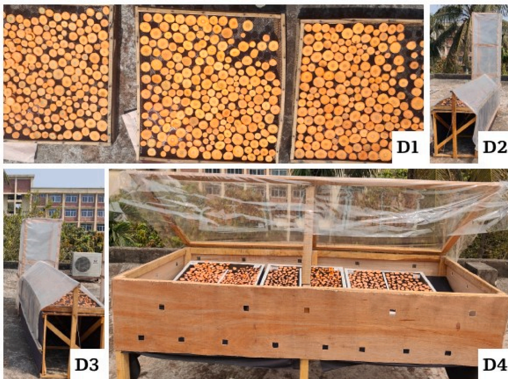
Fig. 1. Different types of solar dryers; D1: Open sun drying (OSD), D2: Solar dryer long chimney (SDLC), D3: Solar dryer short chimney (SDSC), D4: Box solar dryer (BSD).
