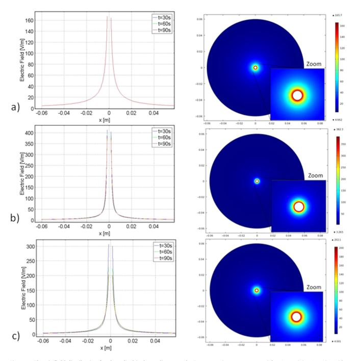
**Figure 8. Electric field distribution for the cylindrical coordinate study.** From top to bottom row: control, freezing and thawing. Aligned for the purpose of comparison. Right column: surface plot. doi:10.1371/journal.pone.0026219.g008
