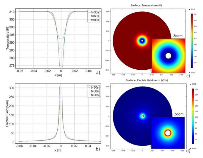
**Figure 6. Data for the cylindrical coordinate study.** The temperature and electric field distribution are illustrated during 90 seconds of thawing. Left column: graph, right column: surface plot. doi:10.1371/journal.pone.0026219.g006
