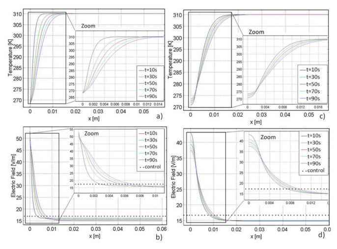
**Figure 3. Graphs for the Cartesian coordinate study.** Left column: temperature and electric field distribution during 90 seconds of freezing. Right column: temperature and electric field distribution during 90 seconds of thawing. Each line represents a 20 second time increment. The dotted line shows the electric field in tissue held constant at body temperature for the same voltage boundary conditions. doi:10.1371/journal.pone.0026219.g003
