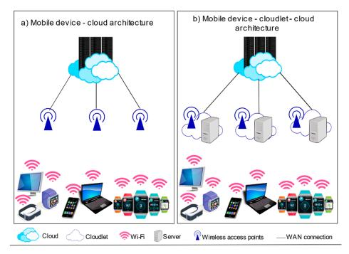
Figure 6. Mobile device-cloudlet-cloud model.
