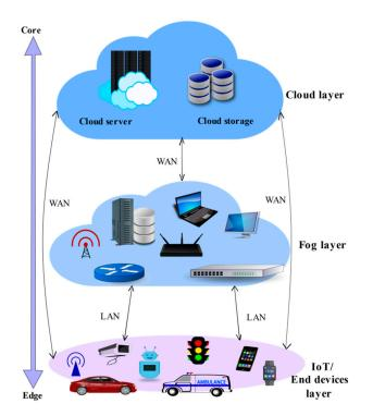
Figure 8. Typical cloud-fog computing architecture.
