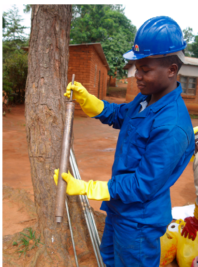
Figure 1. Dynamic cone penetrometer.
