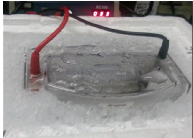
**Figure 7:** Transfer should be done on ice
