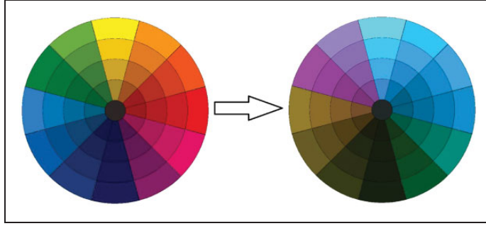
Figure 5. RGB to CIE L*a*b* conversion allows us to manage with color mapping within color frequencies well perceived by color blind people.
