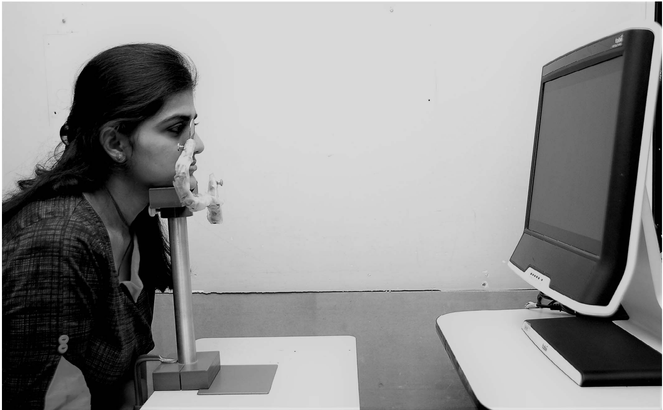
Figure 1. EMP test set up comprising of a 17-in TFT monitor with an inbuilt infrared-based eye tracking camera at the bottom panel . The chin rest placed at a distance of 55 cm was used for each measurement including a PMMA blocker holder positioned in a standard lens holder.
