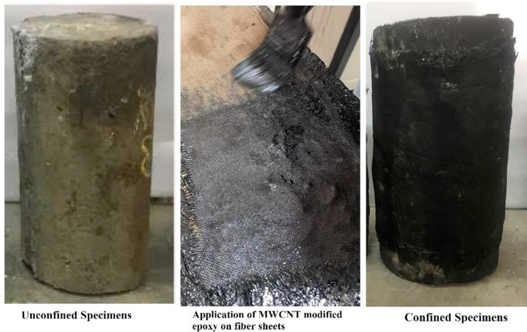
Figure 2. Various stages involved in specimen preparation.
