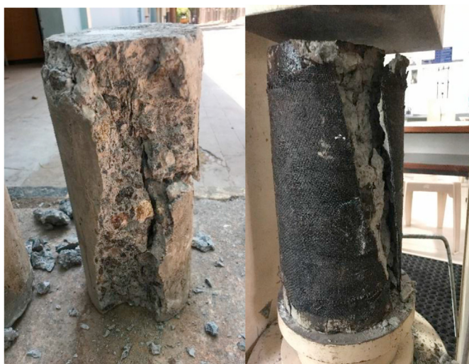
Figure 12. Failure pattern (a) Plain concrete (Control Cylinder) and (b) confined cylinder (C-C1S2B3).
