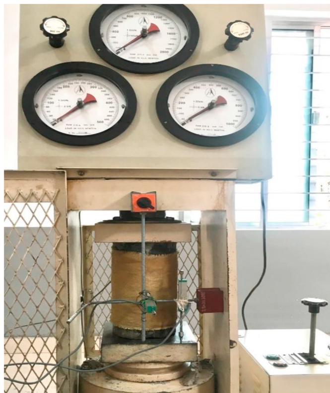
Figure 3. Compression test setup.
