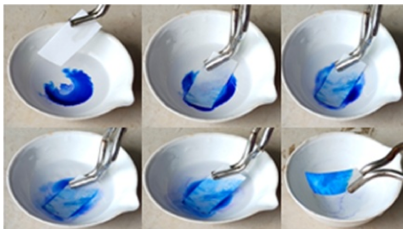
Figure 13. Separation process or absorption of oil from water using CdO-CE (or ST)/PCL-grafted composite-modified cotton fabrics.
