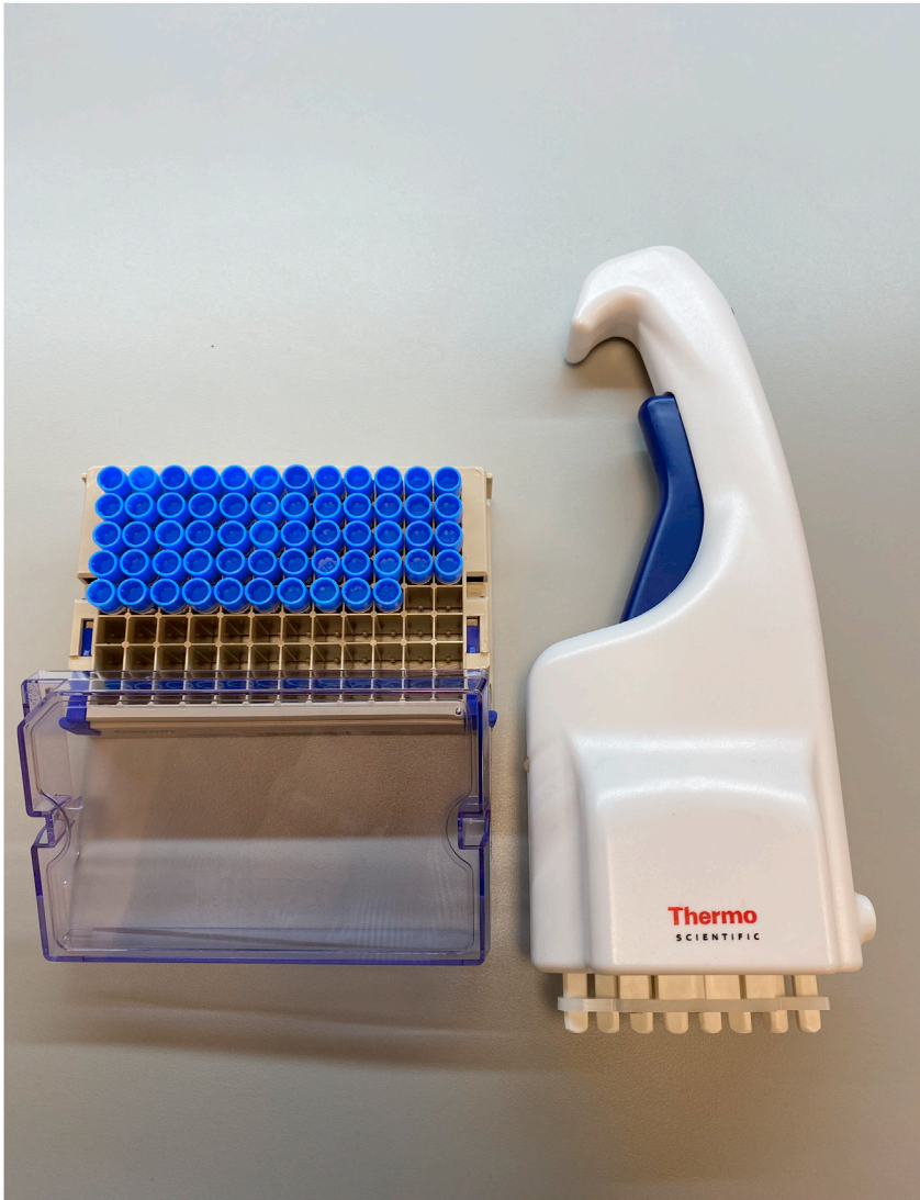
Figure 4. Latch rack for BD® AbSeq Ab-Oligo tubes and 8-channel screw cap tube capper
