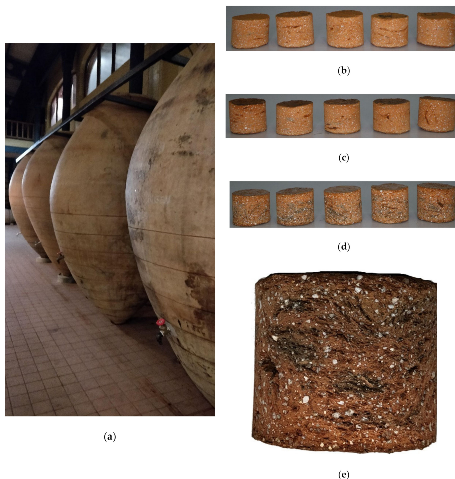
Figure 3. (a) Vessels in Prado Rey winery (Burgos, Spain) and (b) uncoated raw test specimens; (c) specimens coated with 85% colophony + 15% beeswax; (d) specimens coated with 85% beeswax + 15% almond oil and (e) detail of the composition of the vessel wall.
