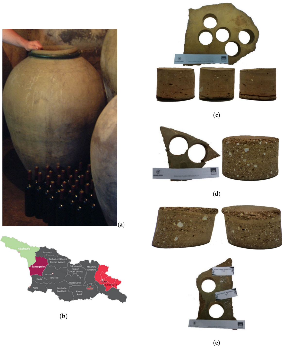
Figure 4. (a) Actual Qvevri vessels; (b) regions of origin of the ceramics tested, Georgia. Vessel pieces and specimens extracted for testing (c) Vardisubani near Telavi (Kaheti); (d) Abkhazia (Makatubani), and (e) Samegrelo.
