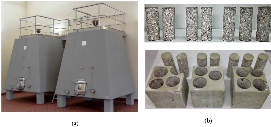
Figure 7. View of (a) concrete tanks (DVTec, France) and (b) pieces extracted for testing next to the concrete blocks supplied.
