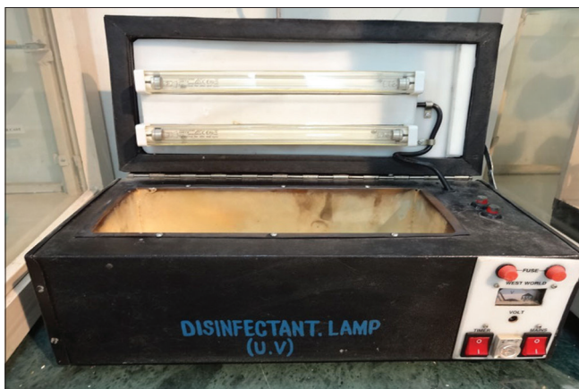
Figure 8: Ultraviolet disinfectant unit
