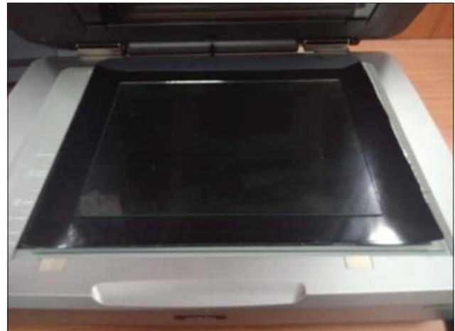
Figure 2: Arrangement to scan the black sheet to measure the  $I_{\text{bckg}}$
