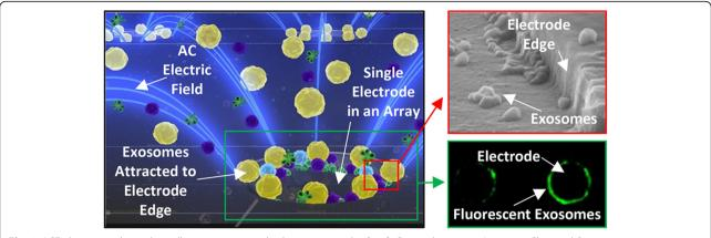
Fig. 3 ACE chip microelectrodes collect exosomes and other microvesicles [104]. Copyright© 2017, American Chemical Society
