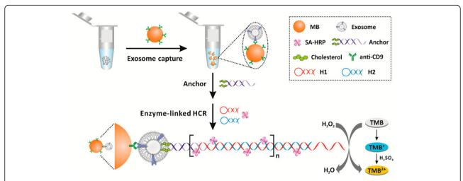
**Fig. 4** Exosome quantification by a method based on immunoaffinity separation combined with cholesterol signal amplification [135]. Copyright© 2017, American Chemical Society
