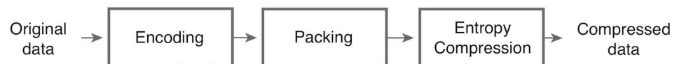
Fig 5. Data flow through compression algorithms. Original data are 3D coordinates of macromolecular structure. At the encoding step the coordinates are transformed to smaller values using one of the encoding algorithms described in this section. Packing converts integer values to a sequence of bytes optimizing the number of bits used to store each value. Entropy compression reduces the syntactic redundancy in encoded data representing by shorter codes symbols that occur more frequently.
