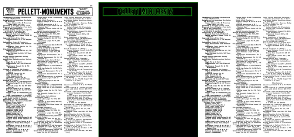
Fig 1. An example city directory page showing the ad removal process. The first panel shows the city directory page as a binary image. The second shows the contours identified as ads by the ad removal algorithm. The final panel shows the image after ad removal.
