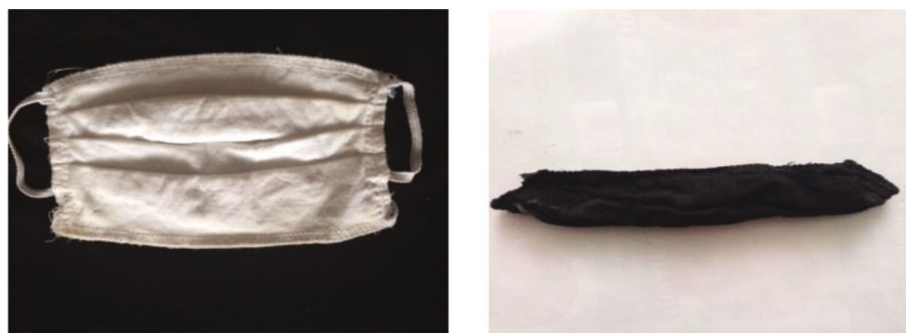
Fig. 7. On the left—used mask of cotton fabric; on the right—the same mask subjected to pyrolysis at T \sim 900^{\circ}\text{C} in cylindrical applicator.
