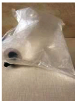
Fig. 8. Thin-film ballast vessel filled with sterile gas.
