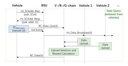
Figure 4. Data query initiated by a vehicle.
