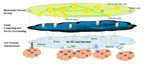
Figure 1. The ITS architecture with blockchain overlay.
