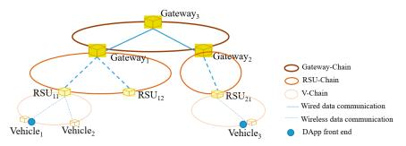
Figure 6. Topology of a vehicular network with ten blockchain nodes.
